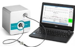
Compact in design, the Flow-UV from Uniqsis sets a benchmark for real time monitoring of continuous flow and batch applications. Unlike many UV-visible spectrophotometers the high-resolution Flow-UV CCD array detector does not require calibration or routine servicing. The Xenon flash lamp source used in the Flow-UV has a lifetime of up to 10 years.
